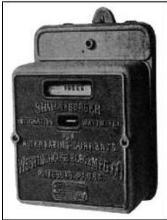
Shallenberger's integration wattmeter, 1894
