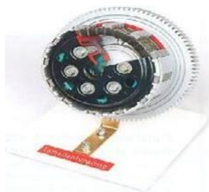
Fig: Cutaway Model Of Multi-Plate Clutch
