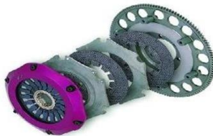
Fig: Exploded View Of Multi-Plate Clutch
