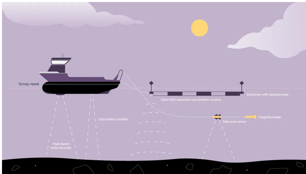
Εικόνα 2.4 Έρευνα HRG ( https://us.orsted.com/renewable-energy-solutions/offshore-wind/offshore-wind-farm-construction/offshore-site-investigations )
