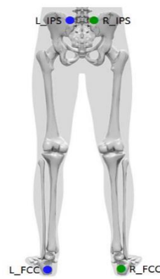
Figure 3. Lower Body marker locations, dorsal view. External markers were used to obtain 3-D joint kinematic data.
