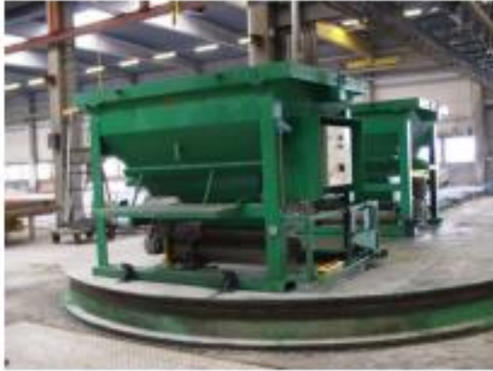
Figure 12.1 Use of an auger holding tank/hopper to activate the SCC just prior to placing.
