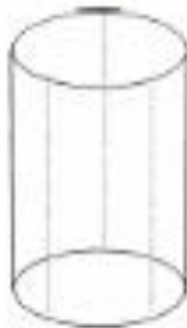
Figure B.3 — Dotted lines showing the measuring positions for the ends of a cylinder
