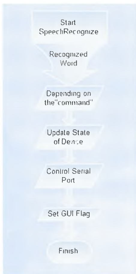
Figure 4.5 – Flow diagram of SpeechRecognized
