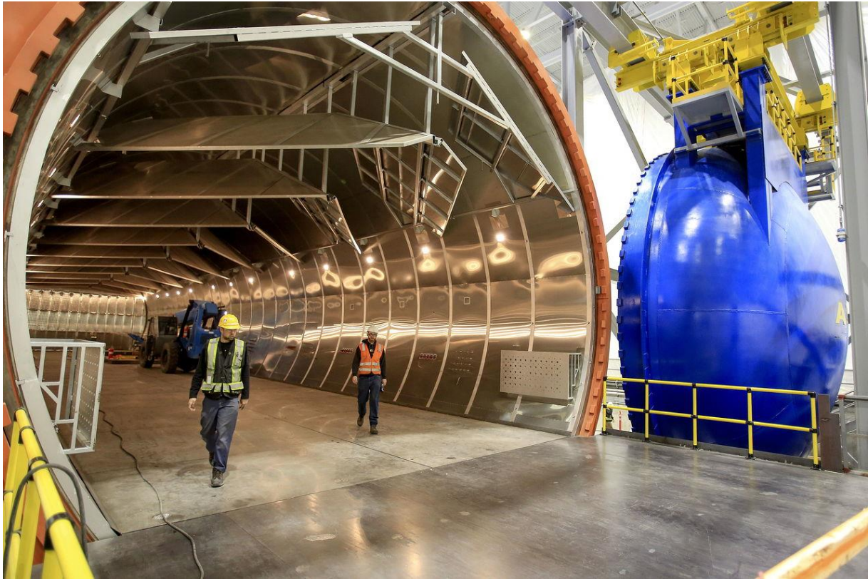
Εικόνα 2.18: Autoclave at the new 777X composite wing center, Everett Washington. [3]
