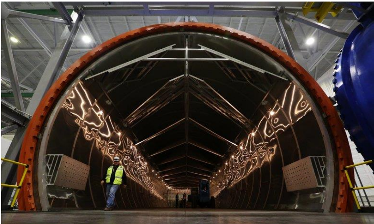
Εικόνα 2.19: Autoclave at the new 777X composite wing center, Everett Washington. [3]
